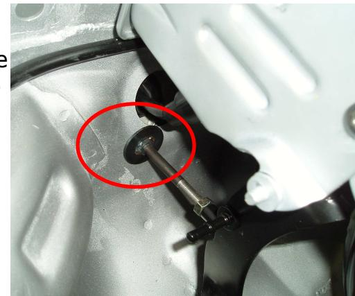
**Nota :** during an adjustment of the clutch free play in service or at the workshop, it is also advised to check if the position of the limit stop is functional. In the contrary case, readjust it.
